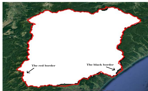
Fig. 5. Compare of the watershed boundaries created by ArcGIS and IFAS (The red border is made with ArcGIS, Drainage area: 8997km2)
